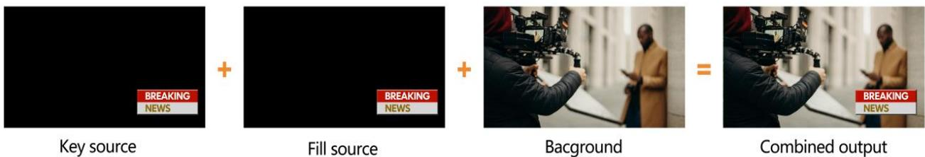
Downstream keys are the last layer of keying and operate independently of the selected "background." No matter what operation is performed on the switch, the overlaid downstream key will remain on the screen. Downstream keys are very suitable for displaying logos on the screen.
