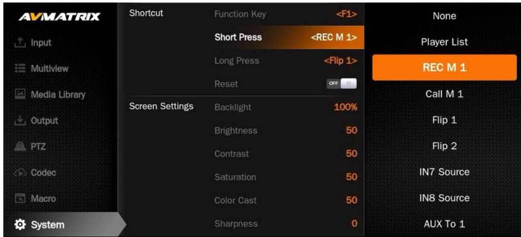
In the macro menu, the user can select for each macro either a single pass mode (execute once and stop) or a cyclic mode (cycle through until manually stopped). Up to 20 macro scripts can be stored locally and can be configured with shortcut keys for quick recall.
