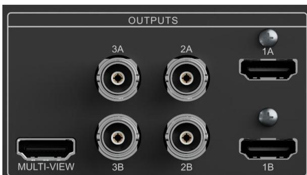
Note: The A/B interface outputs are two connectors of the same signal.
