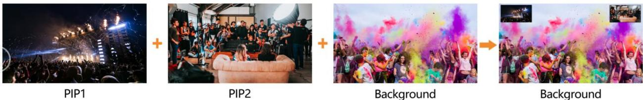
The video switcher supports three groups of PIP. When the corresponding button is pressed, a small image will appear in the upper left corner of the PVW window. Press the menu knob or directly operate on the keyboard panel to select the PIP settings interface. Users can set the size, position, key source, border, color, etc., of the PIP. Press the ON AIR button next to the corresponding button to make the PIP on PGM take effect. PIP
