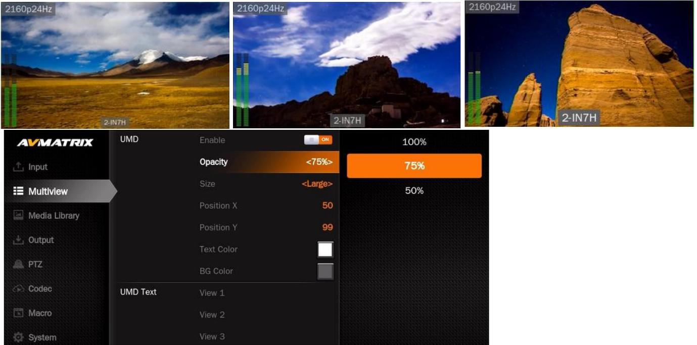
The character content of the screen labels can be set from the menu. Users can rename the label character content for each screen window through a virtual keyboard and the rotation button. Up to 7 characters of label content are supported. The default label format is the screen number-input interface style. For example, 2-IN2 means that the second screen displays the image from input 2. Labels can be customized according to actual scenarios, such as "telephoto position" or "wide-angle position."
