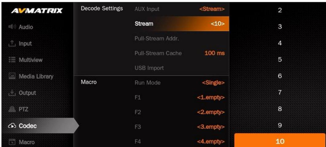
The following configuration presets 10 pull-stream addresses, supporting HTTP/RTSP/RTP/MMS/TS/SMB, etc.
