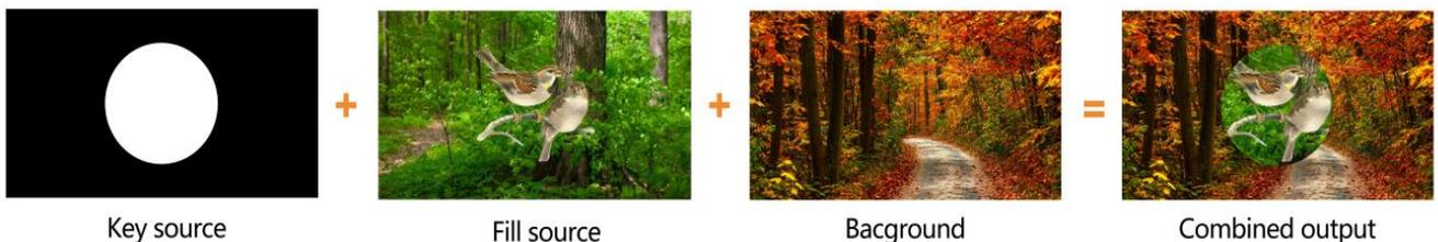
The luma key provides a method for compositing text clips on a background clip based on the brightness levels in the video. Turn on the luma key and adjust the appropriate brightness threshold. Parts of the key source image with brightness values lower than the set threshold will be removed,
