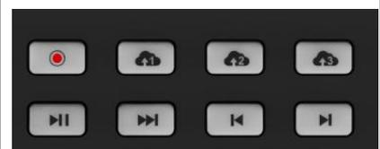
Streaming: Press to start and stop streaming on three preset streaming platforms. Flashes when connected, stays on during streaming, and turns off when stopped.
