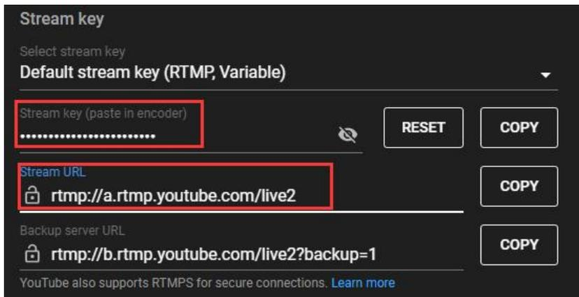
**Steps 4:** Open the streaming settings, and users can select the desired streaming platform. After selecting the streaming platform, paste the streaming key into the specified field. Enable the "start streaming" option to start the live broadcast. If the desired streaming platform is not in the menu, users can select the custom mode.
