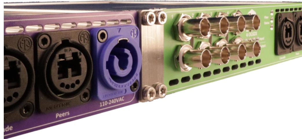
2 units interlocked. Ready for rack mounting
