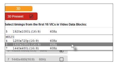
4. Specify the transmission format of the 3D video data, near the bottom of the page.
